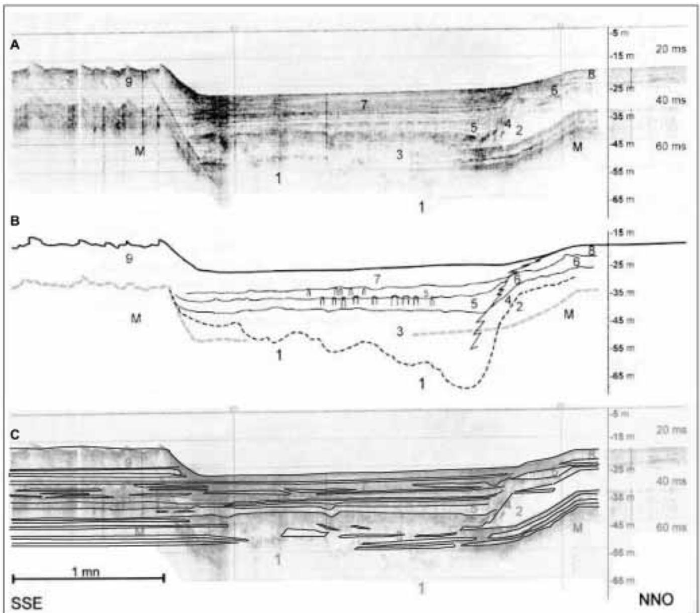
Fig. 2 - The seismic profile (A) located to the south of La Playa beach ridge (Fig.1) used by ORRÙ *et al.* (2004) to establish an unconformity between Holocene and Tyrrhenian deposits (B). Interlayering is evident in our interpretation (C).
