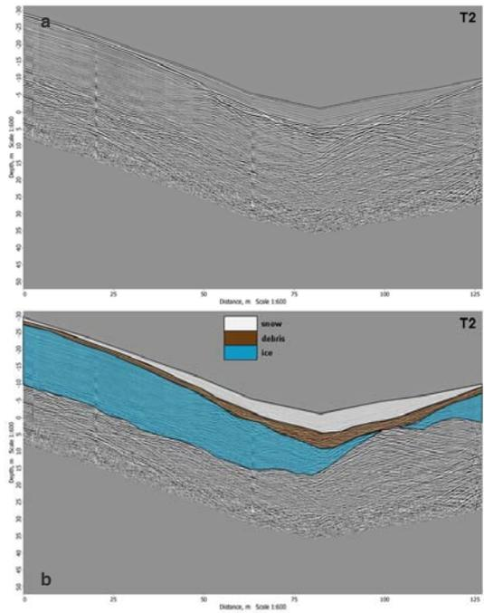
Fig. 6- Georadar scan section T2 (a) and the same section with the units enhanced using different colours (b).
