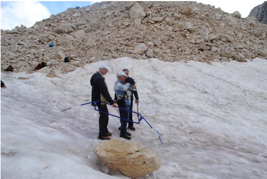
Fig.2 - The used GPR system: unshielded antenna and acquisition unit. Firn covers debris (T1 scan).
