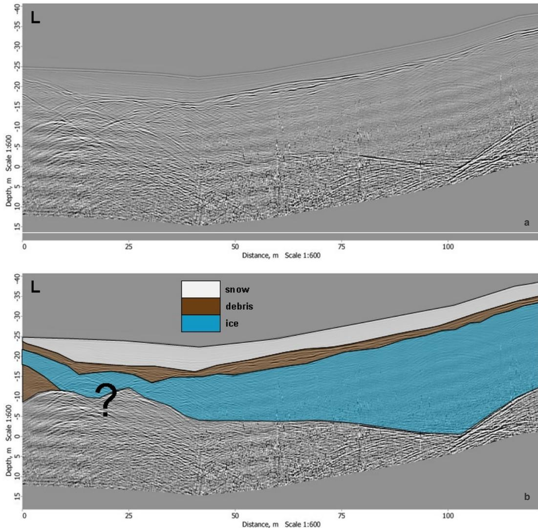
Fig. 4 - Georadar scan section L (a) and the same section with the units enhanced using different colours (b) .
