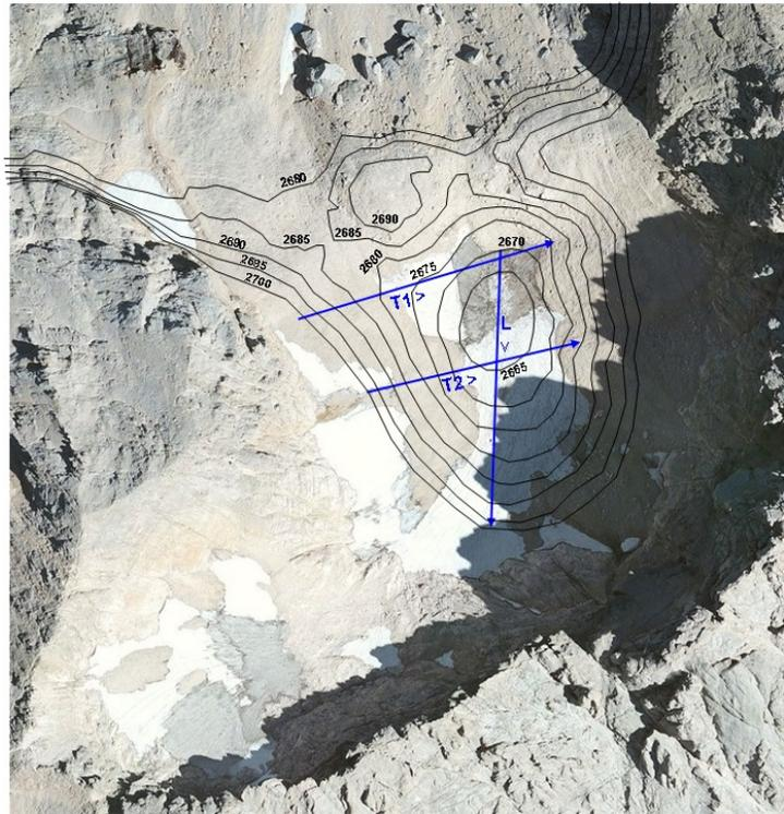
Fig.3 - The Calderone Glacier: aero-photographic image with contour levels and scan sections.
