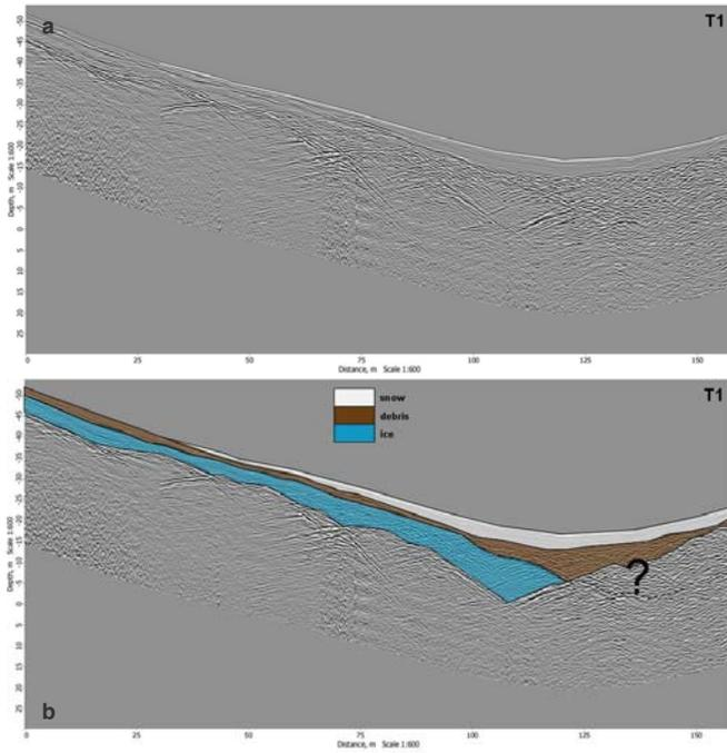
Fig. 5 - Georadar scan section T1 (a) and the same section with the units enhanced using different colours (b).
