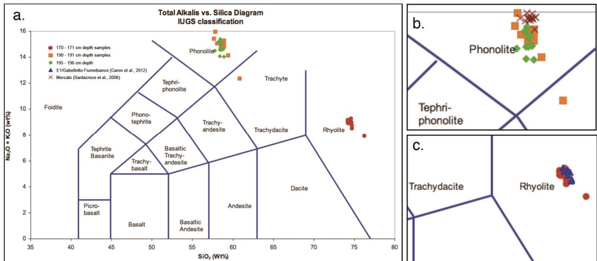
Fig. 5 - Total Alkali-  $\text{SiO}_2$  diagram (Le Bas et al., 1986) for the studied tephra layers (a); Comparison with layers at 190-191 and 195-196 cm with Mercato chemical data (Caron, 2009; Caron et al., 2012) (b); Comparison with E1/Gabellotto-Fiamebianco tephra layers (Caron et al., 2012).
