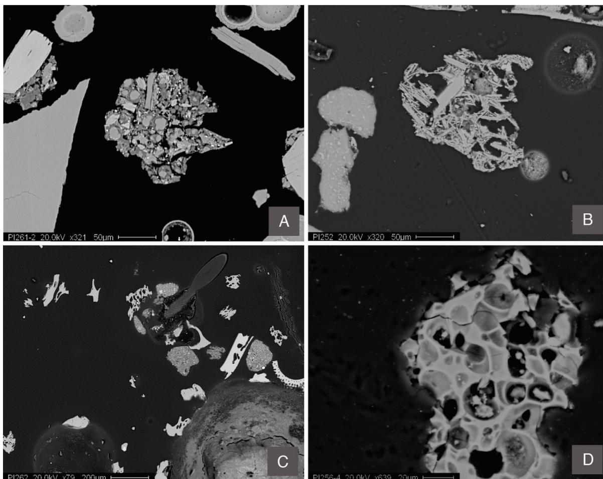
Fig. 3 -Tephra morphology by SEM-EDS. (A) Layer 0-1 cm, (B) layer 40-41, (C) layer 170-171 cm and (D) layer 190/195 cm depth.
